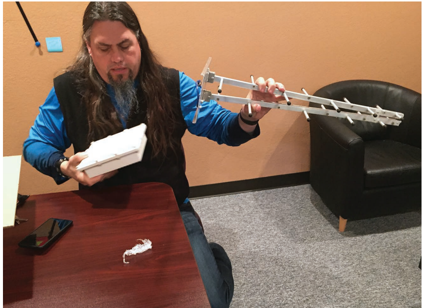
FIGURE 1. Matt Rantanen of Tribal Digital Village (TDV) holds television white space (TVWS) equipment, which is regulated by the US Federal Communications Commission (FCC). The FCC limits both the height above average terrain (HAAT) and power levels at which transmission equipment can be operated, which affect the distance the signals can travel.
